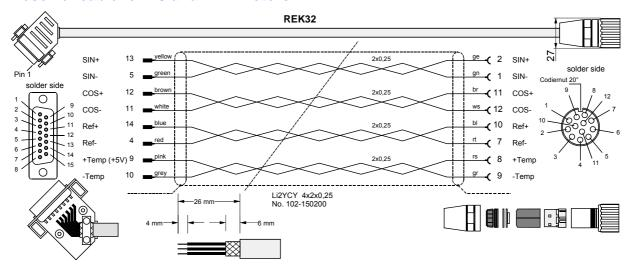
In HJ – motors, ensure that the thermal sensor has the correct terminal arrangement.
